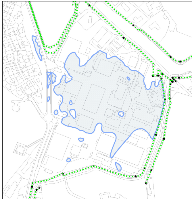
Figure 23 - 1 in 200yr surface water flooding extent, Vector Aerospace
