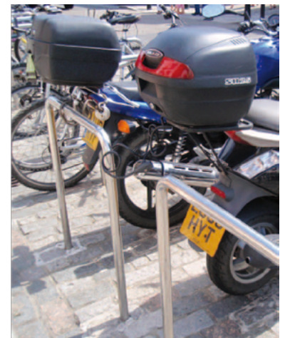
Note: cobbles are not appropriate surface treatment for PTW parking
