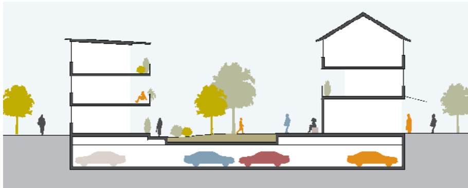
Underground parking with communal space above
