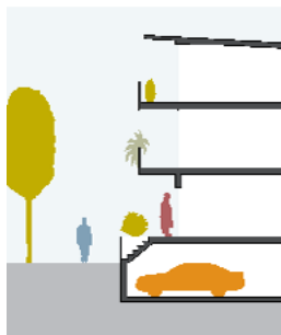
Partial underground parking with raised floor
