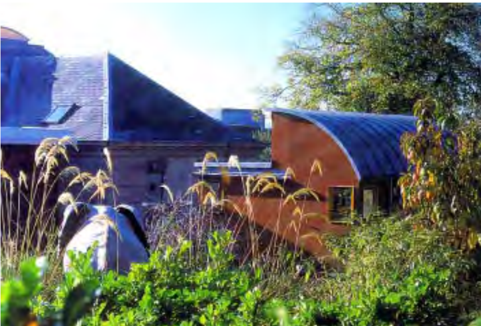
Marketing suite for Edinburgh Zoo, showing successful use of curved metal roofing and coloured roughcast on a business building, adjacent to an older structure. Architect: Smith Scott Mullan
