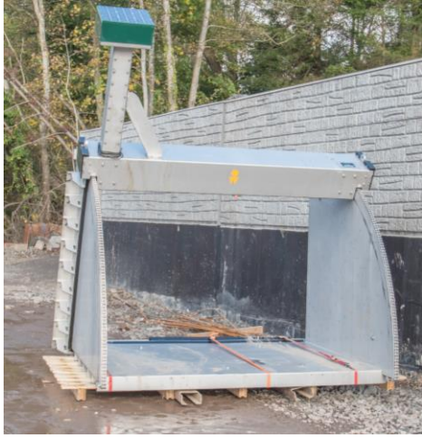
75. Trout Farm – Tilting Weir (this structure will control flow from the Lade into Trout Farm).
