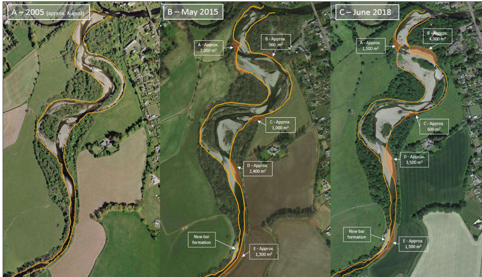
Figure 3-1: Satellite images from Google Earth showing channel change between 2005 and 2018. The 2005 bank lines are shown in orange on all images.
