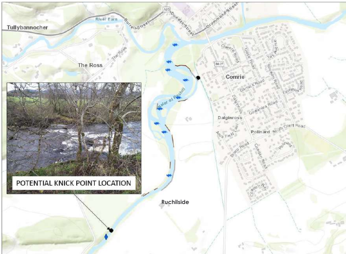
Figure 3-12: Map showing the potential location of the knick point where it appears to have stabilised against bedrock. A drop in bed elevation was observed.
