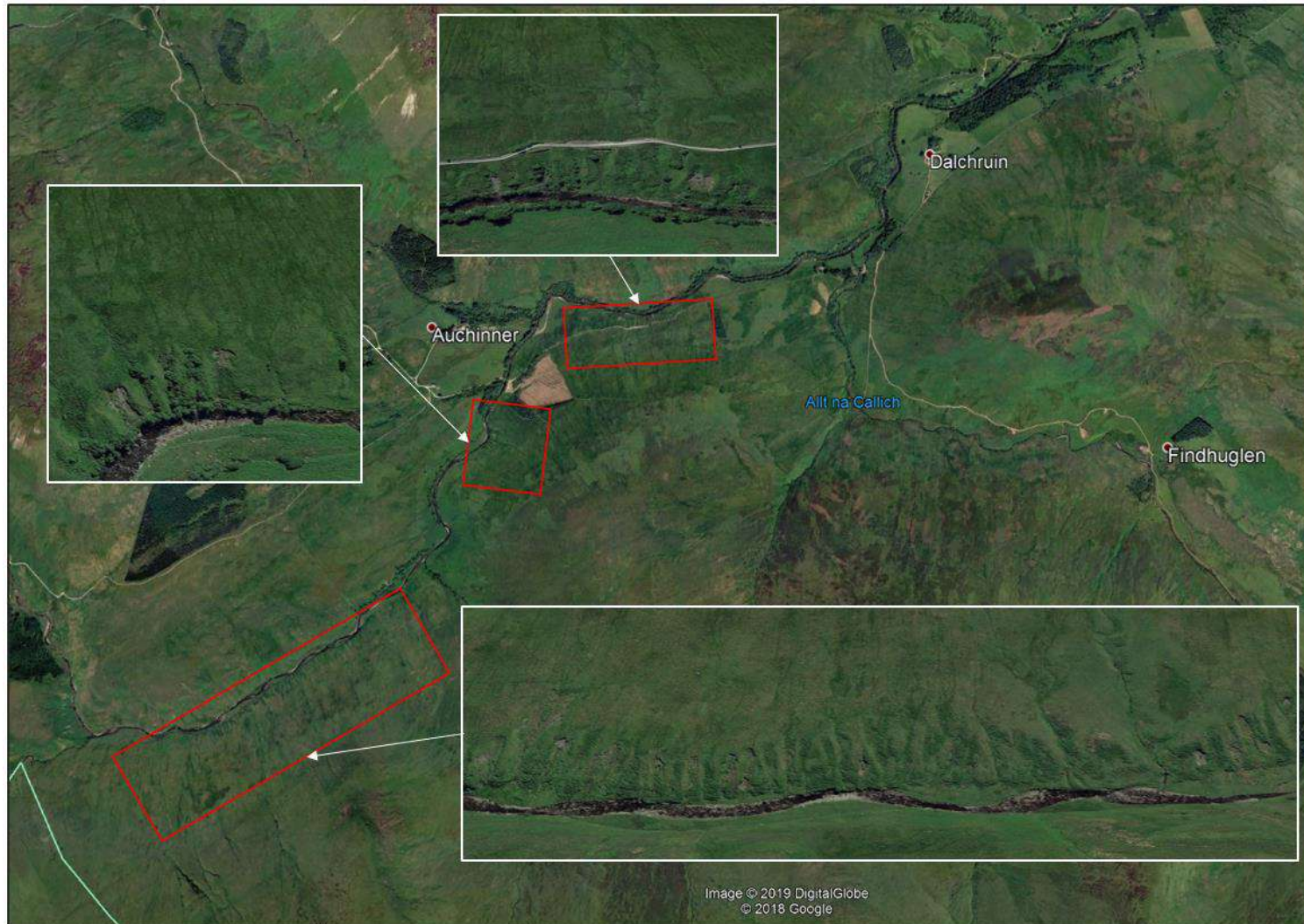
Figure 3-4: Google Earth image showing areas of gully erosion which appear to have resulted from changes to drainage patterns from upslope peat drainage.
