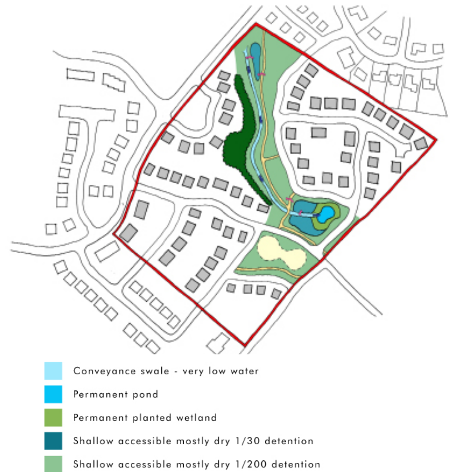
Figure 2 – Example of integrated SuDS (PKC Open Space Provision for New Developments supplementary Guidance 2021)
