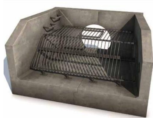
Figure 12 Typical Headwall and trash screen
