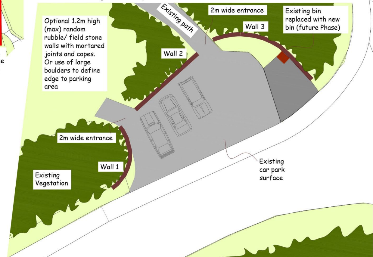
Sketch Plan Showing Outline Proposals at Eastern Car Park and Path to Kinnoull Hill
