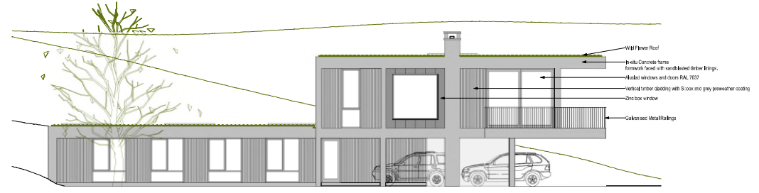
NORTH WEST ELEVATION
